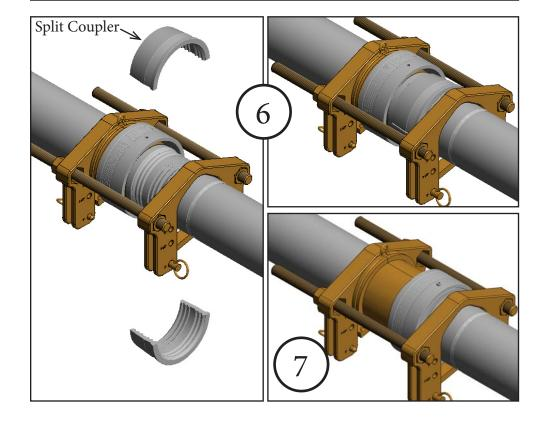
6. Install both halves of DOL split couplers and slide retaining ring into place. 7. Install set screws to secure coupling 8. Dis-assemble clamp in reverse order to remove.
