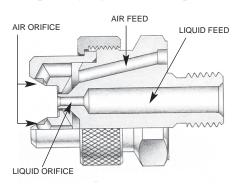
**Cutaway View: External Mix Set-up**
