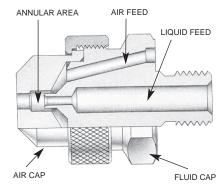
Cutaway View: Internal Mix Set-up
