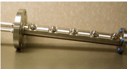
Simple piping and robust design describe this multiple nozzle XA lance.
