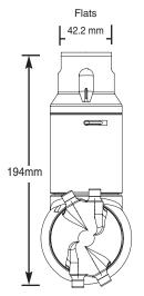
Vertical Nozzle Head Alignment Clearance Diameter: 85 mm
