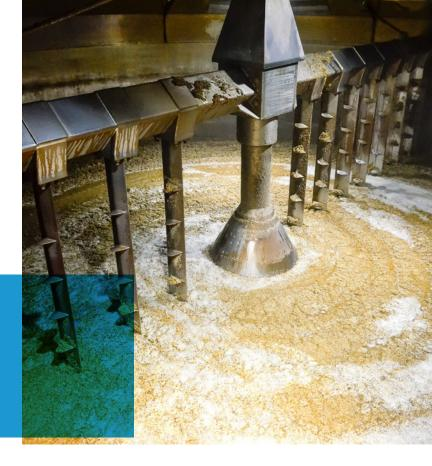
In the lautering process, spent grains and husks often find their way into the cleaning process's recirculated water. These particulates tend to clog and plug standard spray devices for tank cleaning, which becomes a maintenance nightmare for any brewer.
