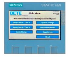
A touchscreen Human Machine Interface (HMI) allows users to configure the spray system and adjust spray parameters through an easy-to-navigate menu of options. Adjustable parameters for each spray zone include nozzle cycle rate, duty cycle, trigger signal delays, and trigger state.
