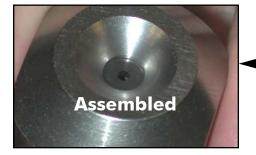
The carrier need only be HAND TIGHTENED, DO NOT WRENCH TIGHTEN! Check to see that the orifice is seated against the inside of the carrier.
