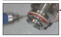
Apply lube to the o-ring on the body before installing into the carrier (We do not want the o-ring to stick to the carrier when it is being threaded on).
