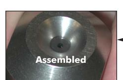
Apply lube to the o-ring on the body before installing into the carrier (We do not want the o-ring to stick to the carrier when it is being threaded on).
