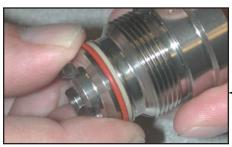
Install a new o-ring on the body by rolling it over the end and into the groove (DO NOT start part of the o-ring into the groove and stretch it over the end. Doing this stretches the o-ring and can nick or damage it). Caution: DO NOT use screwdrivers, utility knives, etc. to remove o-ring from the body. Use no metal tools, they can nick or damage the body.
