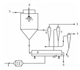
Two Stage Dryer with Vibrating Bed Dryer Fig. 2.8.2
