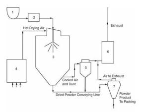
Open Cycle Co-current Flow Layout Fig 2.4.1
