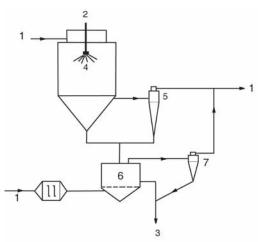
Two Stage Dryer with Fluid Bed Dryer Fig. 2.8.1
