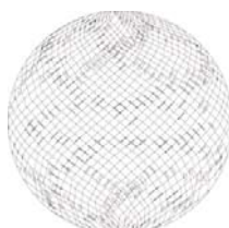
Orbitor 4 nozzle spray pattern
