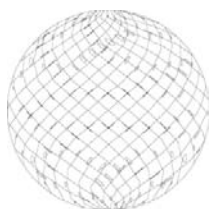
Orbitor 2 nozzle spray pattern
